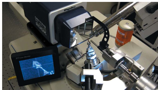
Figure 5 A typical X-ray diffractometer setup with a cryosystem. At the center is a crystal mounted on a pin magnetically held on a goniometer head. Clockwise from lower right corner: X-ray source collimator pointing towards the crystal with X-ray beamstop; black microscope; microscope display of the crystal in the cross-hairs mounted in a loop; X-ray detector; cryosystem nozzle pointing at the crystal; orange X-ray shutter indicator lamp. Note that the cryonozzle is pointing obliquely at the sample position so that the cryogenic gas impinges neither on the goniometer head nor on the X-ray detector, nor does it obscure the view of the crystal through the microscope.
