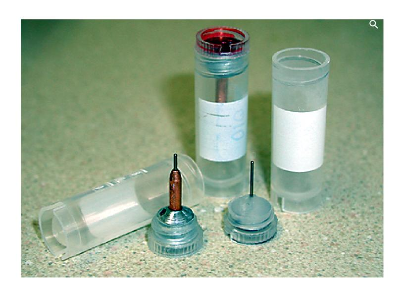
Figure 1. Mounting loops and cryovials
