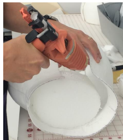
Fig. 6 Glue the Ethafoam® to the interior of the Fosshape® form
