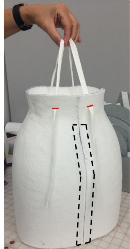
Fig. 7 A strip of blueboard (black dashed line) is glued to the interior of the form to close the center back seam and twill tape is threaded through slits in the Fosshape® (red lines).
